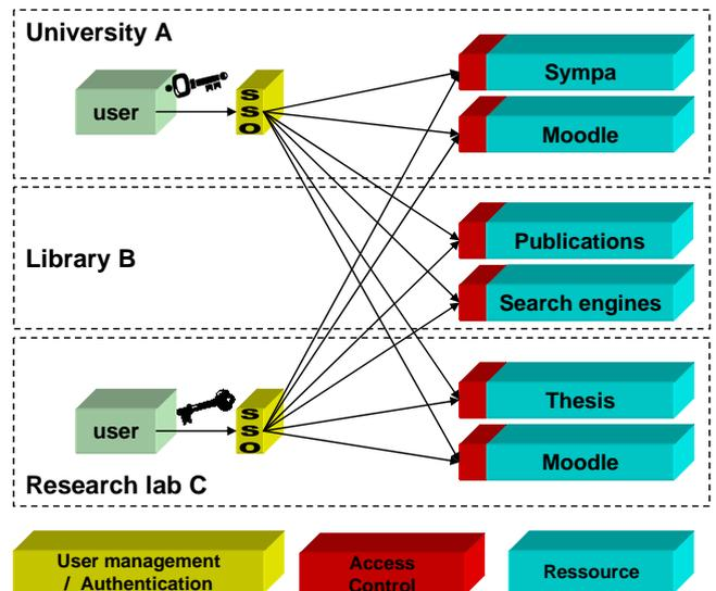
Figure 2 – Sharing web resources with Identity Federation (inspired by Switch AAI)
