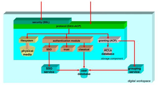
Figure 3: Software architecture
